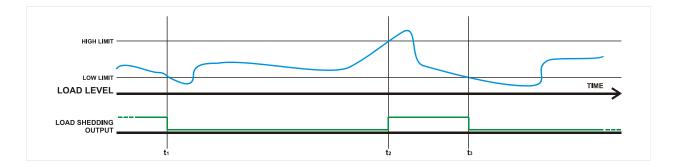
t1: the load goes below the Load Shedding Low Limit, thus the Load Shedding output becomes inactive.
