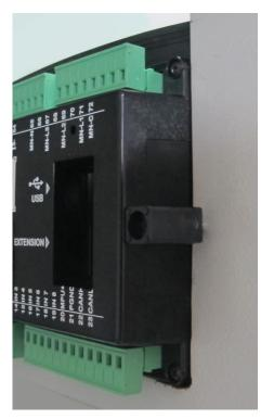
Installation of screw type bracket
