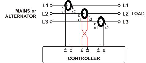
The generator is still loaded with 100 kW On each phase. The load Power Factor (PF) is 1. PF in phase L2 will show -1,00 due to reverse CT polarity. The result is that total generator power displayed by the controller is 100 kW.
