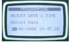
These parameters allow adjusting the battery backup real time clock of the module. Once set, the clock will continue to run even if DC power is removed from the unit.
