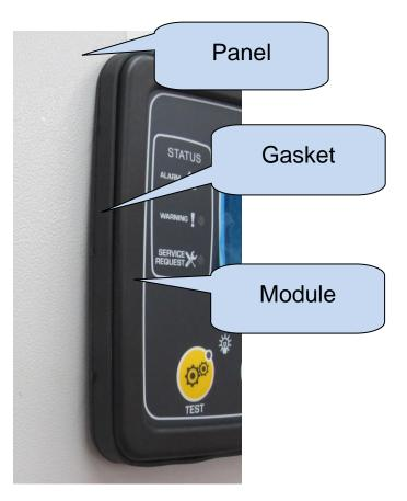
The rubber gasket provides a watertight means of mounting the module to the genset panel. Together with the gasket, IEC 60529-IP65 protection can be reached from the front panel. A short definition of IP protection levels is given below.
