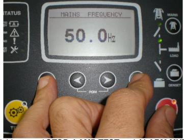
Hold pressed STOP, LAMP TEST and ALARM MUTE
