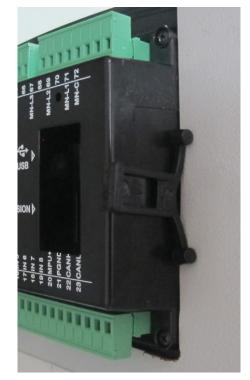
Installation of self retaining type bracket
