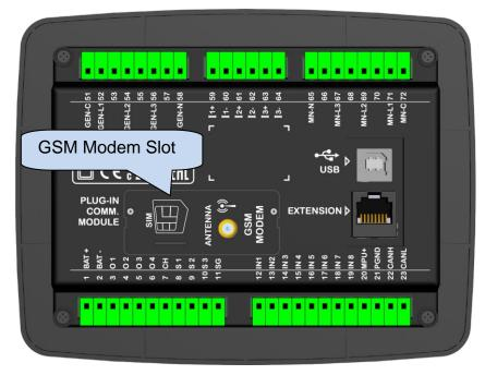
The module requires a GPRS enabled SIM card for full functionality. Voice-only type SIM cards will usually not function properly.
