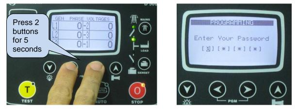
Skip the password entry screen by pressing the button 4 times. The screen below left will come. Press again the button. The last stored event will open, as in the below-right picture. The first page will display the event number, event type, fault type and date-time information.
