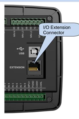
The module provides resources for 32 additional digital inputs and 32 additional digital outputs.
