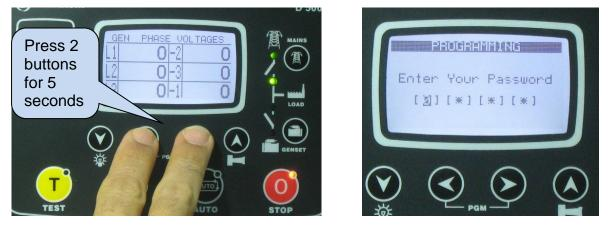
A 4 digit password must be entered using **O O O** buttons.
