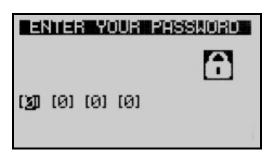
When the configuration mode is entered, the password entry screen will be displayed.
