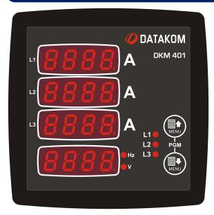
The DKM-401 is a low cost precision instrument designed to display various AC parameters in a 3-phase distribution panel.
