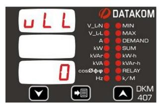
This parameter sets the low limit for low voltage alarm.
