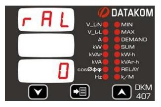
This parameter sets the low limit for low reactive power alarm.
