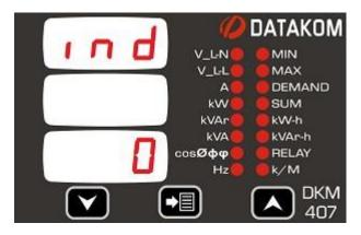
This parameter sets the detection delay of the digital input signal in miliseconds.
