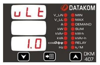
This parameter sets the ratio of voltage transformers.
