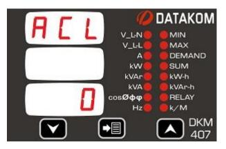
This parameter sets the low limit for low active power alarm.
