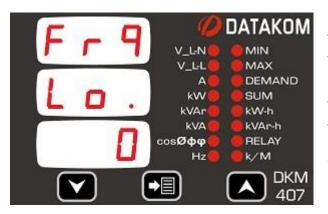
This parameter sets the low limit for low frequency alarm.
