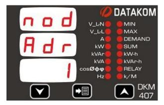
This is the Modbus node address of the device. Each device in a Modbus network must have a different node address.
