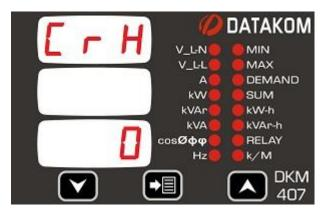
This parameter sets the high limit for overcurrent alarm.
