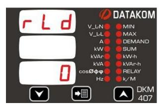
This parameter defines the delay between all conditions are met and the relay operates. (in seconds)
