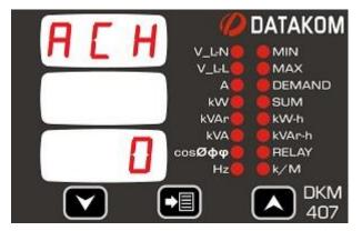
This parameter sets the high limit for excess active power alarm.
