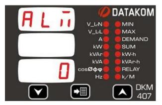
This parameter defines the delay between an alarm condition occurs and the device gives the alarm. It defines also the delay between an alarm condition is removed and the alarm goes off.
