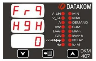
This parameter sets the high limit for high frequency alarm.
