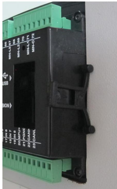
Installation of self retaining type bracket
