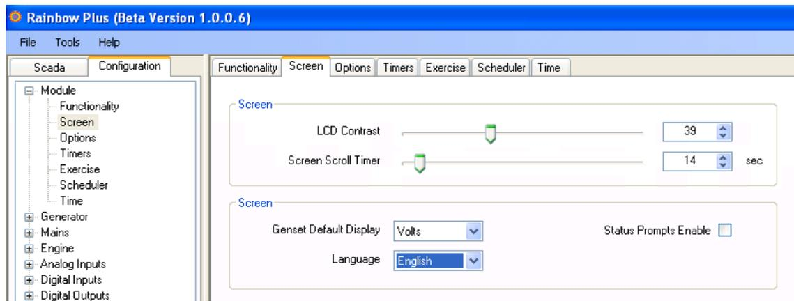
Eventually the same parameter can be modified through the front panel programming menu. The related parameter is Controller **Configuration > Screen Scroll Timer**.
