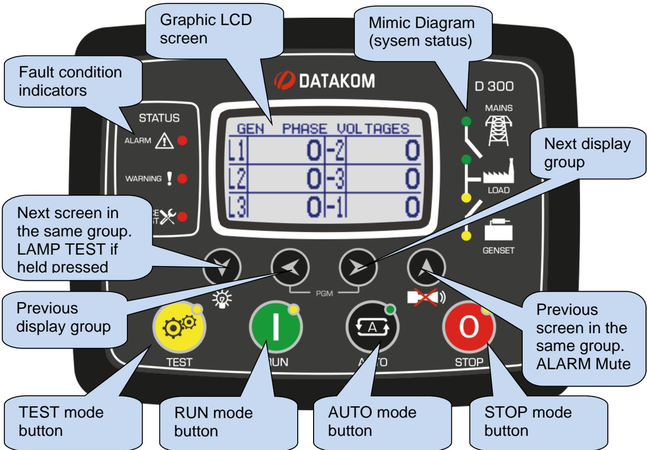
When the engine hours **OR** the time limit is over, the **SERVICE REQUEST** led (red) will start to flash and the service request output function will be active. The service request can also create a fault condition of any level following parameter setting.
