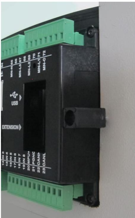
Installation of screw type bracket
