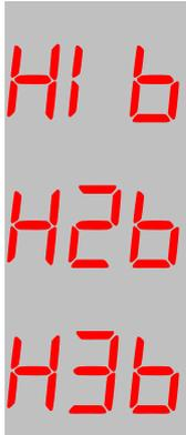
These parameters determine respectively the humidification start lower limits for humidity sensors 1 , 2 and 3.
