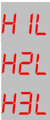
These parameters adjust the low relative humidity alarm limit for the related sensor.
