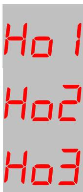
These parameters determine respectively the offset value to be added to relative humidity sensors 1, 2 and 3.
