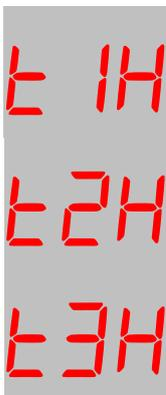
These parameters adjust the high temperature alarm limit for the related sensor.
