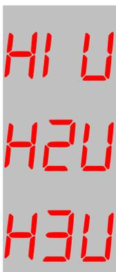
These parameters determine respectively the de-humidification start upper limits for humidity sensors 1 , 2 and 3.
