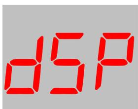
This parameter selects the screen menu where the unit returns when no pushbutton is pressed during 1 minutes.
