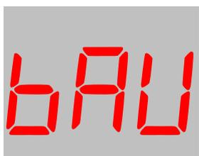
This parameter determines the data rate (baud rate) used in the Modbus communication. Every unit in the same Modbus loop must use the same data rate.
