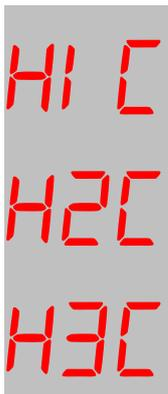
These parameters determine respectively the hysteresis values for stopping the humidification/de-humidification for humidity sensors 1 , 2 and 3.
