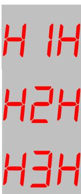
These parameters adjust the high relative humidity alarm limit for the related sensor.
