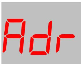
This parameter determines the Modbus node address of the unit. Every unit in the same Modbus loop must have a different node address.
