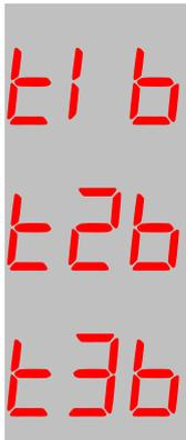
These parameters determine respectively the heating start temperature limits for temperature sensors 1 , 2 and 3.
