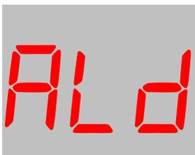
This parameter adjusts the delay for alarm activation after an alarm condition occurs. It also determines the delay for alarm deactivation after the alarm condition is removed.
