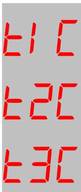
These parameters determine respectively the hysteresis values for stopping the heating or cooling for temperature sensors 1 , 2 and 3.
