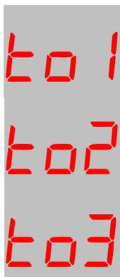
These parameters determine respectively the offset value to be added to temperature sensors 1, 2 and 3.
