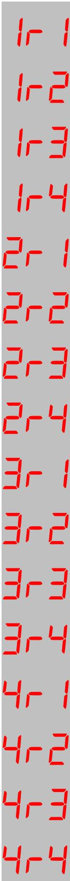
The unit provides 4 relay outputs. Each output reflects the combination of 4 different relay functions. The combination options are explained in the next parameter.
