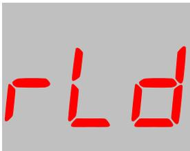
This parameter adjusts the delay for relay activation after all conditions for relay operation are met.
