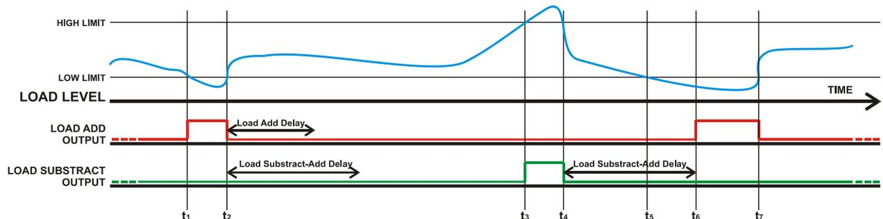
**$t_1$ :** the load goes below the Load Shedding Low Limit, thus the Load Add output becomes active.
