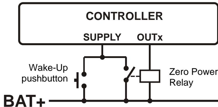
The controller wakes-up on applying the power through the “wake-up” pushbutton. Then it will immediately activate the zero power output which will cause the zero power relay to feed the controller.
