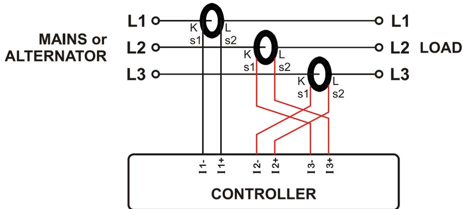
The generator is still loaded with 100 kW on each phase. The load Power Factor (PF) is 1. PF in phases L2 and L3 will show -0.50 due to phase shift between voltages and currents which is caused by CT swapping. The result is that total generator power displayed by controller is 0 kW. Measured values are as follows:
