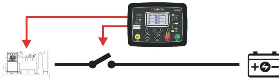
The complete charging cycle will always include a float charge cycle. Following programming, a boost charging cycle may be added.
