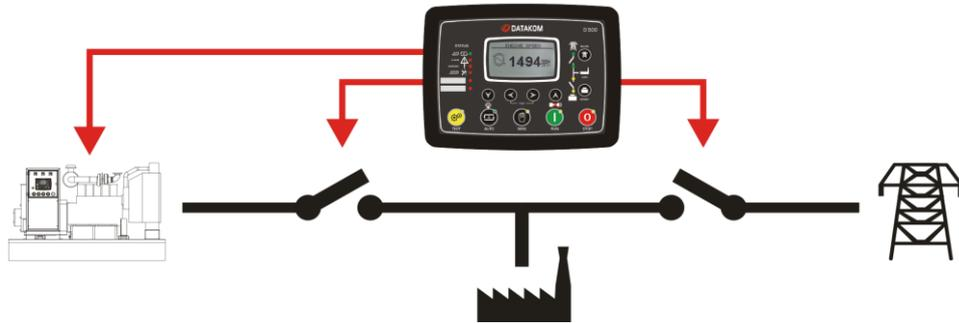
The unit features both MPU and J1939 CANBUS inputs. Thus, both mechanical and electronic engines are supported.
