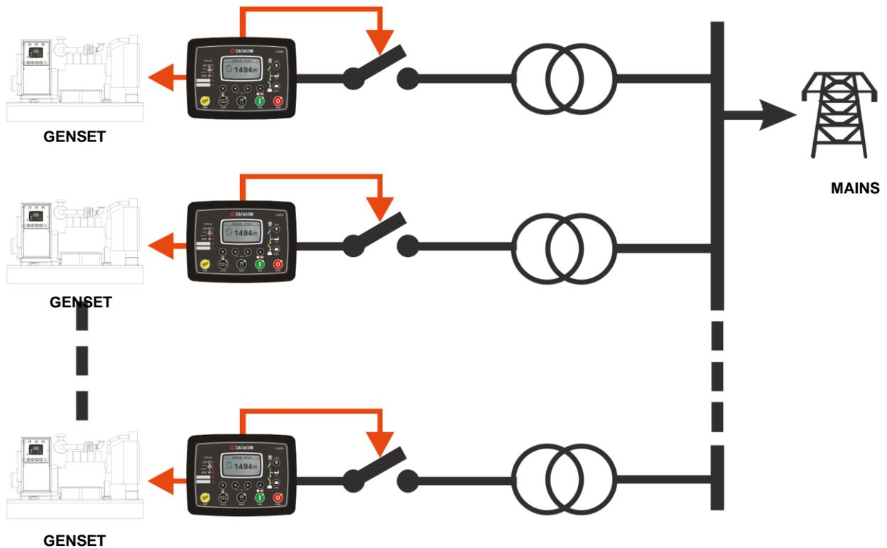
The **Distributed Power Export to Mains** mode allows an unlimited number of gensets to export power to the mains and share active and reactive loads without any communication between controllers.
