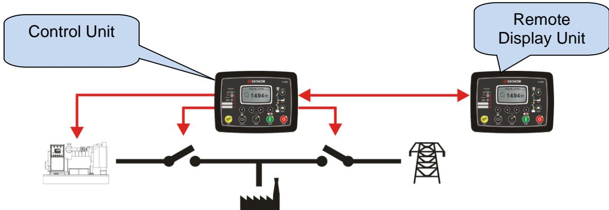
The connection between two modules is done through RS-485 ports. For the best results, a 120 ohms balanced, low capacitance cable should be used.
