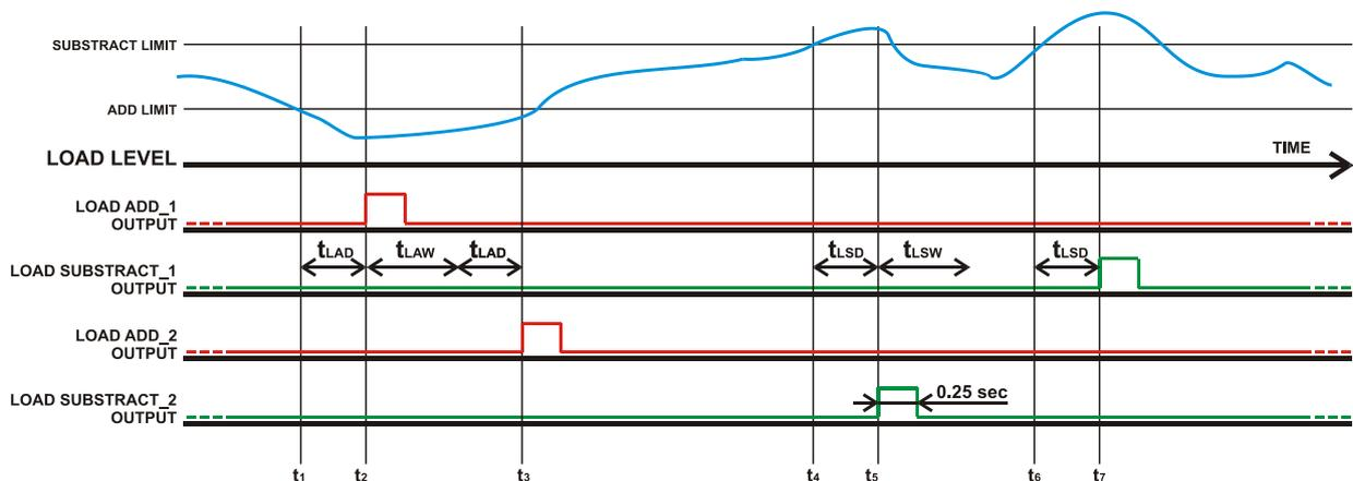
**t<sub>1</sub>:** the load goes below the Multi Load Add Power Level.
