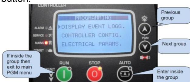
Navigation inside a group is made also with ▼ and ▲ buttons. A list of available parameters will be displayed. Selected parameter is shown in reverse video (blue on white). In order display/change the value of this parameter, please press [PGM] button.
