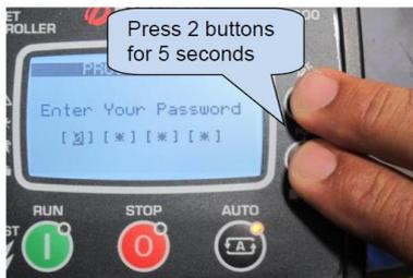
A 4 digit password must be entered using ▼, ▲, [PGM] and [I] buttons.
