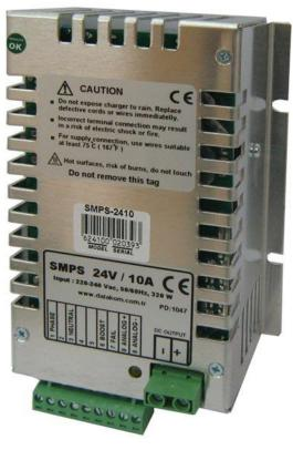
The units provide a "boost charge" input as a standard feature. When this input is pulled to battery negative, the output voltage of the charger will be set to the boost charge voltage. This feature may be used temporarily to improve battery life.
