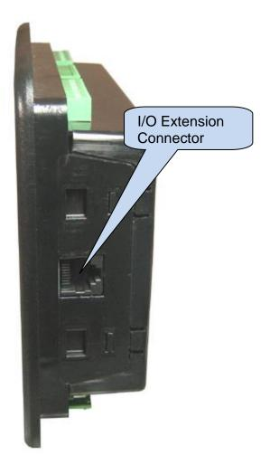
The module provides resources for 32 additional digital inputs and 32 additional digital outputs.
