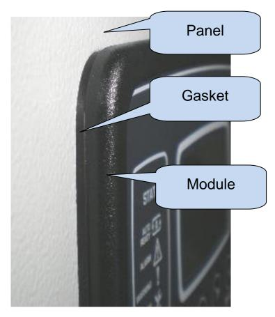
The rubber gasket provides a watertight means of mounting the module to the genset panel. Together with the gasket, IEC 60529-IP65 protection can be reached from the front panel. A short definition of IP protection levels is given below.
