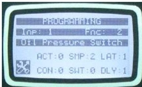
The unit has 5 digital inputs. Only parameters of one input are explained below. Other inputs have identical parameter set.
