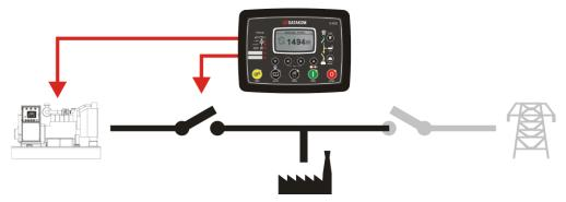
The unit features both MPU and J1939 CANBUS inputs. Thus, both mechanical and electronic engines are supported.
