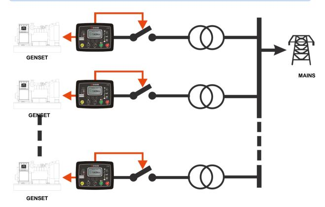
The **Distributed Power Export to Mains** mode allows an <u>unlimited number of gensets</u> to export power to the mains and share active and reactive loads <u>without any communication</u> between controllers.
