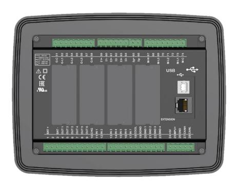
The unit is designed for panel mounting. The user should not be able to access parts of the unit other than the front panel.
