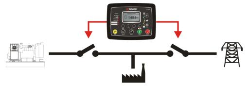
Engine instrumentation and protection will be insured by the engine controller.
