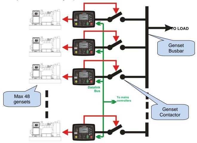
When SYNCH mode is selected, the controller will monitor its REMOTE START input. If the remote start input is active, it will run the genset (depending on settings). The remote start signal is usually provided by a Mains Synchronization unit or an ATS controller. It can be a manually controlled signal as well.
