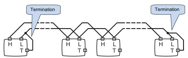
Figure illustrating the Datalink termination from two ends
