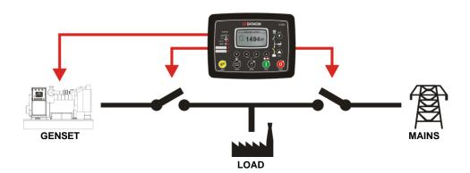
The **Export to Mains** mode allows the multi genset system to supply the mains power grid under constant power factor. Thus the multi genset system will be part of the mains power supply system.
