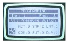
The unit has 8 digital inputs. By using external input expansion modules, up to 40 inputs in total are available.
