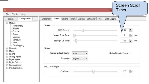
Eventually the same parameter can be modified through the front panel programming menu. The related parameter is **Controller Configuration > Screen Scroll Timer**.
