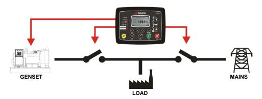
When AMF functionality is selected, there are a number of adjustable parameters causing parallel operation to the grid:
