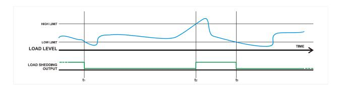
**<u>t1:</u>** the load goes below the Load Shedding Low Limit, thus the Load Shedding output becomes inactive.
